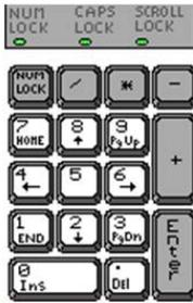
This part of the keyboard can be used to type numbers and the numeric symbols that go along with them. Keep in mind that these numbers and symbols will look and act no differently than the matching numbers and symbols on the typewriter section of the keyboard. It is merely another configuration for the keys for speed of use for those accustomed to using an adding machine or calculator, which has the number keys set up in this same pattern.
